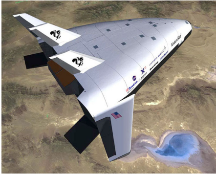
Figure 4.2.1-57. Single-stage-to-orbit (SSTO). Although it never got off the ground as shown in this artist's conception, the X-33 program pioneered many key technologies. They may one day help us build an efficient rocket that uses a single stage to orbit. (Courtesy of NASA/Marshall Space Flight Center)
