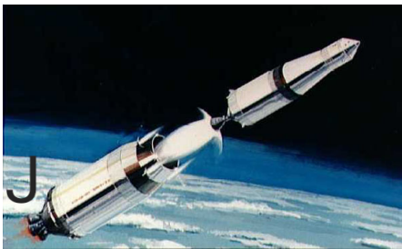
Figure 4.2.1-56. Saturn I during Staging. When a launch vehicle, such as the Saturn I shown here in an artist's concept, stages, it shuts off the lower-stage rocket, separates it, and ignites the rocket on the next stage to continue into orbit. (Courtesy of NASA/Kennedy Space Center)
