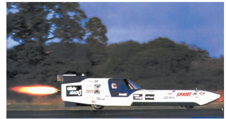
Figure 4.2.1-29. Maximum Impulse! The Gillette Mach 3 Challenger used HTP/HTPB hybrid motors producing more than 10,000 N (2248 lb.) thrust to reach a peak speed of 365 m.p.h. in an effort to set the world two-wheeled speed record. (Courtesy of Richard Brown, Project Machinery)
