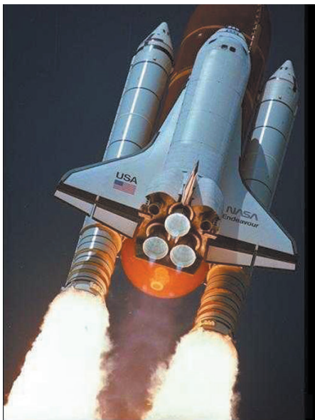
Figure 4.2.1-21. Chemical Rockets. Chemical rockets use the energy stored in the propellants. The Space Shuttle's main engines and solid-rocket boosters are two examples of chemical rockets. (Courtesy of NASA/Johnson Space Center)
