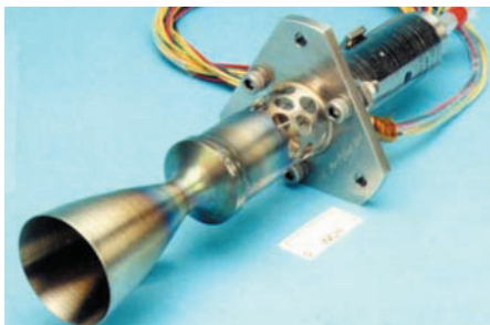
Figure 4.2.1-24. Monopropellant Rocket. This 22 N (5 lbf) hydrazine monopropellant engine built by Kaiser-Marquardt delivers 235 s specific impulse. At only 20 cm (8 in.) long by 4 cm (1.5 in.) wide, it can be easily integrated into a variety of spacecraft for attitude control and small orbital maneuvers. (Courtesy of Kaiser-Marquardt)
