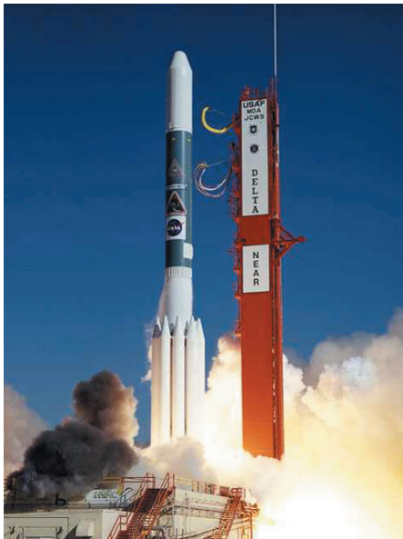
Figure 4.2.1-27. Solid-rocket Boosters. Many launch vehicles, such as the Delta II shown here, rely on solid-rocket motors to get them off the ground. (Courtesy of NASA/ Marshall Space Flight Center)
