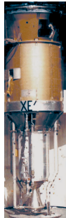
Figure 4.2.1-36. Nuclear Engine for Rocket Vehicle Applications (NERVA) Rocket. The NERVA program tested nuclear-thermal rockets from 1947 until 1972. Future missions may depend on their impressive performance to take humans to Mars. (Courtesy of the Report of the Synthesis Group on America’s Space Exploration Initiative)
