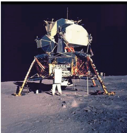
Figure 4.2.1-51. Throttle Back for Landing. The Lunar Excursion Module (LEM) used a throttleable bipropellant engine, allowing the astronauts to control their descent to the lunar surface. (Courtesy of NASA/Johnson Space Center)
