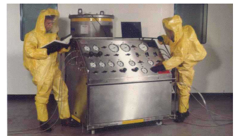
Figure 4.2.1-42. Propellant Loading Operations. Transferring toxic propellants from storage containers to rocket tanks is dangerous and requires safety suits with breathing apparatus and special handling equipment. (Courtesy of British Aerospace Royal Ordnance)
