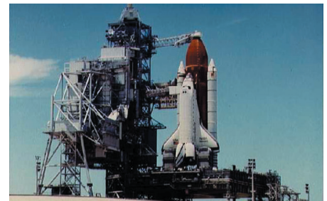
Figure 4.2.1-19. Keeping Things Cool. Cryogenic propellants, such as liquid oxygen and liquid hydrogen on the Shuttle, must remain hundreds of degrees below zero. The cap on the top of the main tank helps control propellant boil off. (Courtesy of NASA/Johnson Space Center)
