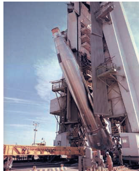
Figure 4.2.1-54. Atlas Inflated for Launch. To provide structural rigidity on the Atlas launch vehicle, the thin aluminum skin of the propellant tanks were inflated like balloons. (Courtesy of the U.S. Air Force)
