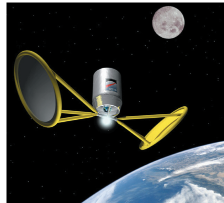
Figure 4.2.1-30. Solar-thermal Rocket. This solar-thermal rocket concentrates solar energy on a thermal mass that reaches very high temperature (up to 2400 K). In this concept, liquid hydrogen flows through the thermal mass, absorbing the energy and then expanding through a nozzle, producing a thrust of more than 6 N (1.6 lbf) at an I_{sp} of 750 s. (Courtesy of NASA/Marshall Space Flight Center)
